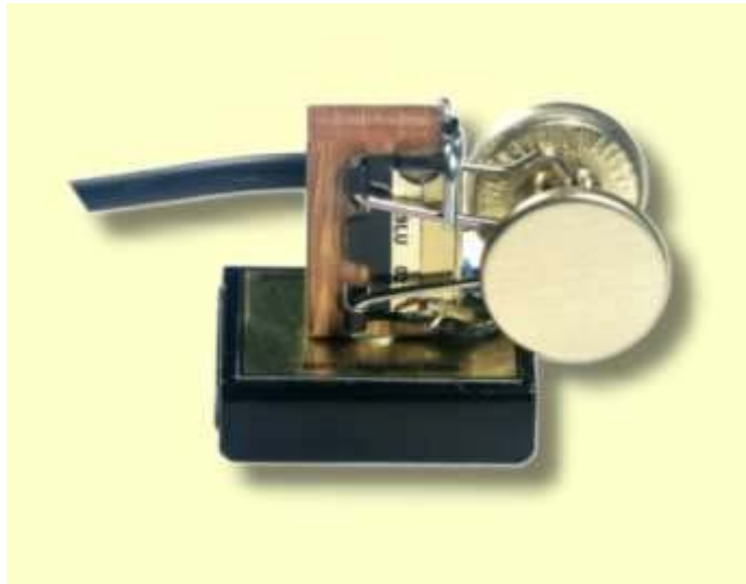
BullDog lambic paddles made from a large paper clip. Make one yourself or buy it from BullDog lambic Keys: http://www.amateurradioproducts.com/bd2.html
