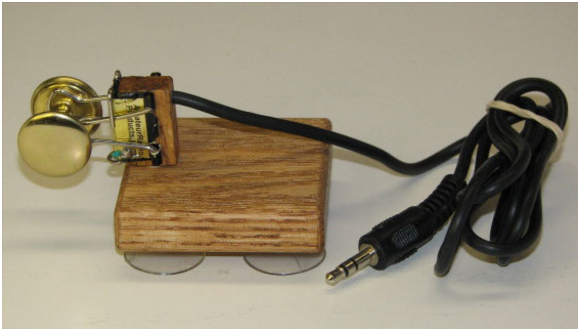
The Bulldog paddle made from a paperclip These are available at http://www.amateurradioproducts.com/
